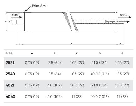
Each element comes packaged with a brine seal and interconnector kit (o-rings installed)
